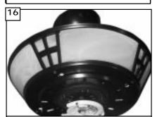
Hang assembled fan from the mounting bracket installed to ceiling. Make sure the fan is hanging straight. Rotate fan until the tab on the Mounting bracket engages the slot on the Downrod Ball. This must be done to prevent the fan body from rotating when the blades are in motion.
